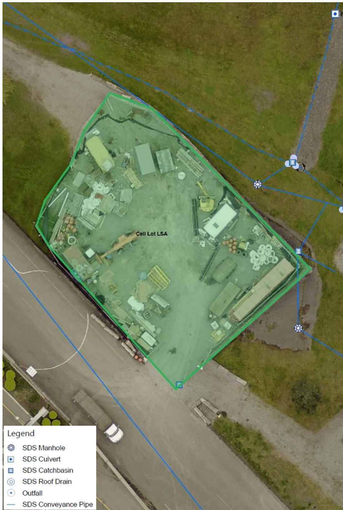
Figure 5. Cell Lot LSA Drainage Details
