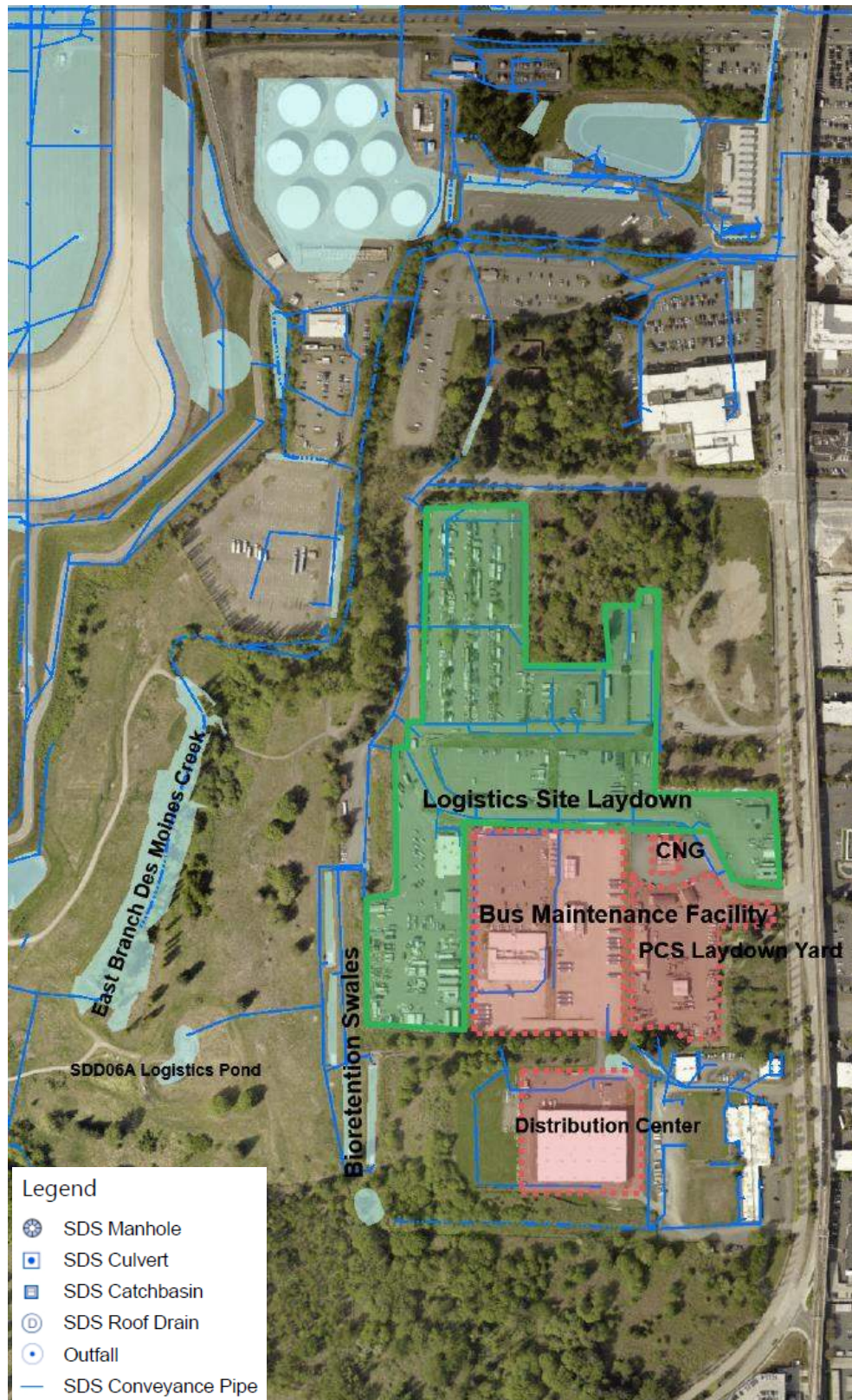
Figure 2. Logistics LSA Drainage Details
